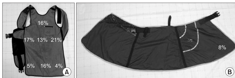
Fig. 4. Defects in the shields are found using fluoroscopic images. The most common site of damage to the radiation-protective shields was at the waist of the aprons (51%) [51]. (A) One-piece-type apron and (B) skirt-type apron. Adapted from the article of Ryu et al. (Korean J Pain 2013; 26: 142-7) [51].
