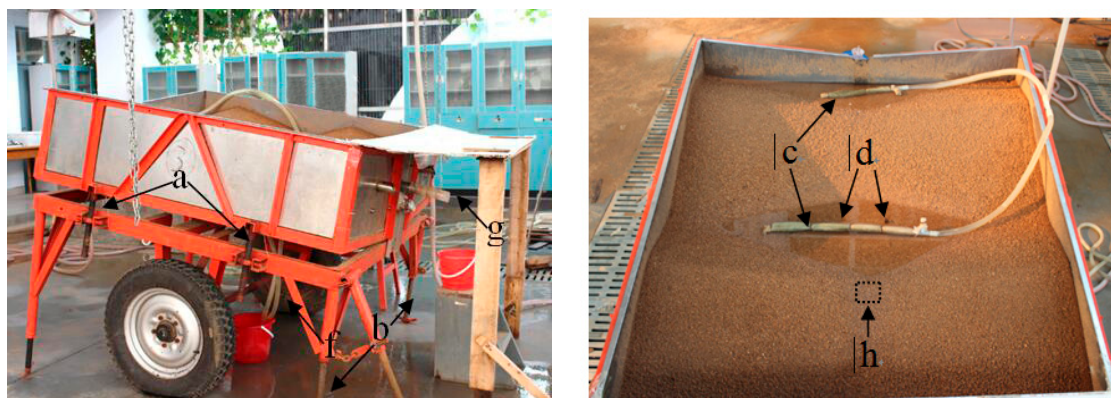
Figure 2. Experimental plot for adjusting row grade and field slope simultaneously by rotating a screw (a) and (b), and creating seepage condition by supplying water with a flow rate of 3 L \text{min}^{-1} to the furrows where the water level was controlled by pipes (d). a, screw for adjusting row grade; b, screw for adjusting field slope; c, pipes for supplying water; d, pipes for adjusting the water level 1 cm lower than the concave spot at the ridge (h); f, pipes for redundant water collection; g, outlet for collecting seepage and surface runoff.
