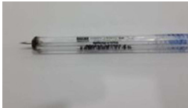
Figure 1 Sharp metal pin used to mark the orientation grooves on resin blocks.
