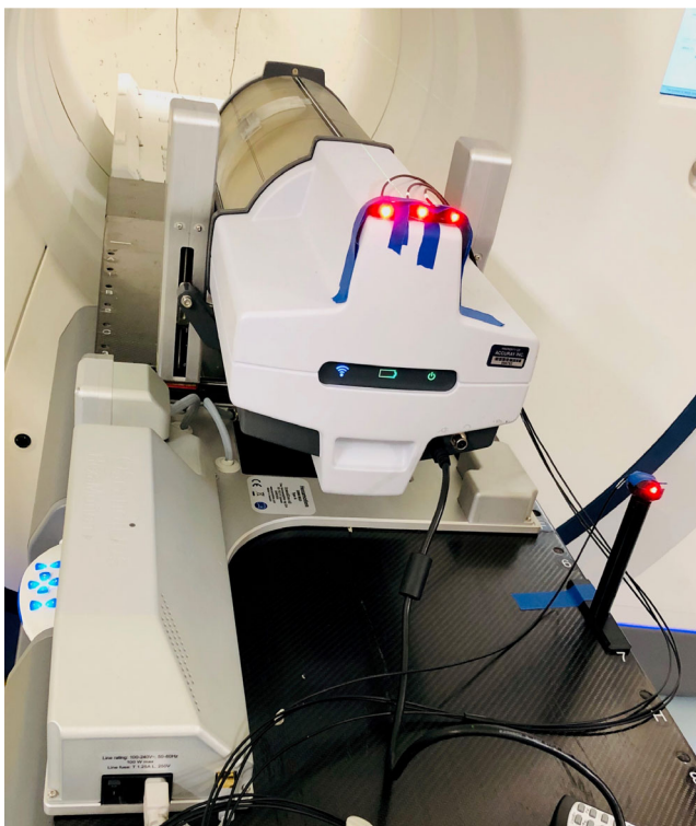
FIG. 3. Delivery setup with Delta4 Phantom + on a HexaMotion six-dimensional motion management system. [Color figure can be viewed at wileyonlinelibrary.com ]
