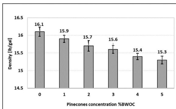
Fig. 9. The density of cement slurry at different concentrations of APCP.
