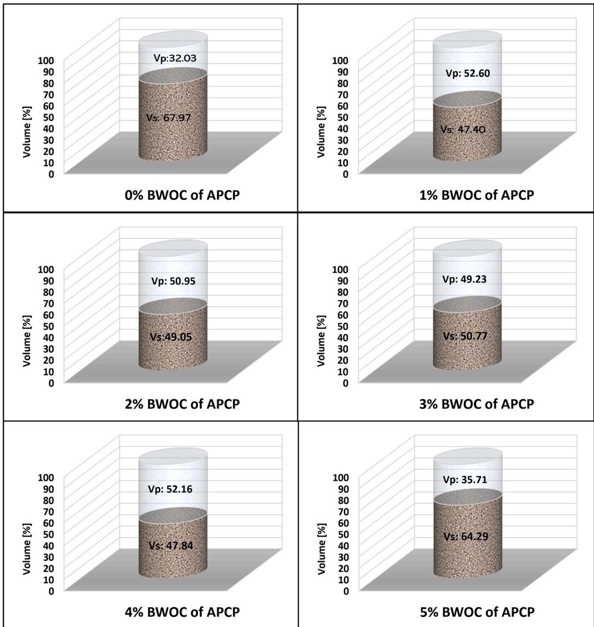
**Fig. 11.** The ratio of solid volume ( $v_s$ ) to void volume ( $v_p$ ) for solid cement samples after adding (a) 0%BWOC of APCP, (b) 1%BWOC of APCP, (c) 2%BWOC of APCP, (d) 3%BWOC of APCP, (e) 4%BWOC of APCP, and (f) 5%BWOC of APCP.
