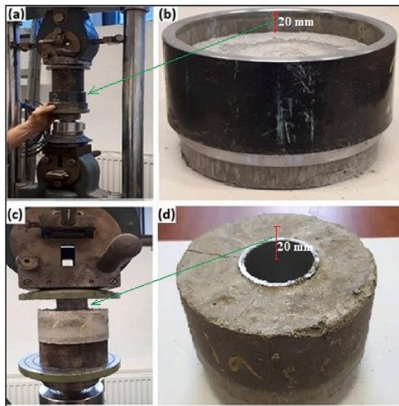
Fig. 21. Interfacial bonding shear strength sample for the first case (a)during and (b) after testing, and for the second case (c)during and (d) after testing.
