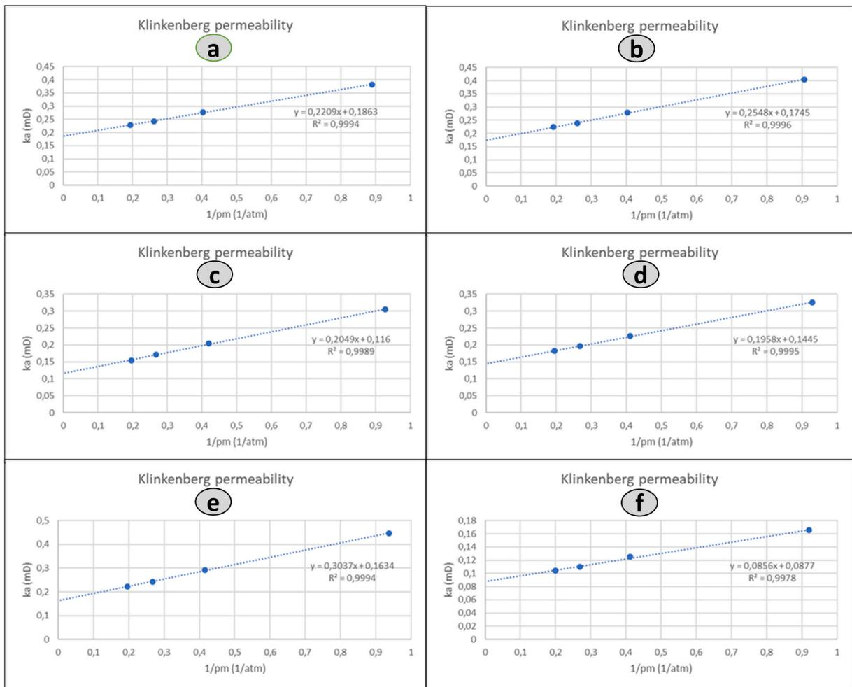
**Fig. 12.** The change in permeability as a function of mean nitrogen pressure for solid cement samples after adding (a) 0 %BWOC of APCP, (b) 1 % BWOC of APCP, (c) 2 %BWOC of APCP, (d) 3 %BWOC of APCP, (e) 4 %BWOC of APCP, and (f) 5 %BWOC of APCP.
