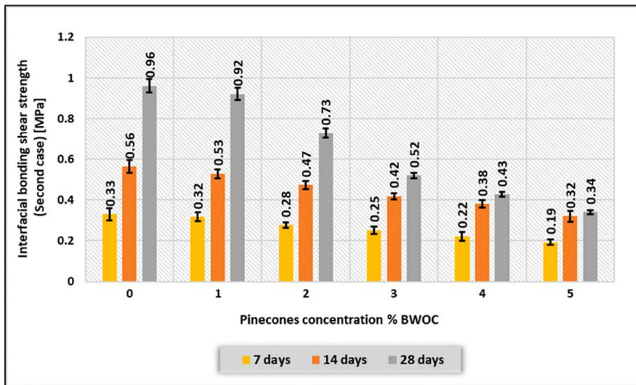
Fig. 20. Interfacial bonding shear strength of the cement samples at different concentrations of APCP for second case.
