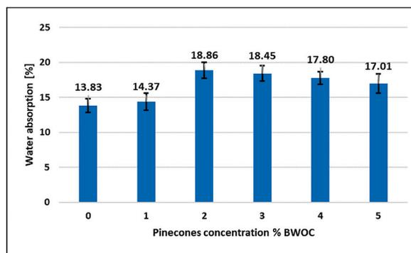
**Fig. 13.** Water absorption results with the addition of increasing concentrations of APCP.
