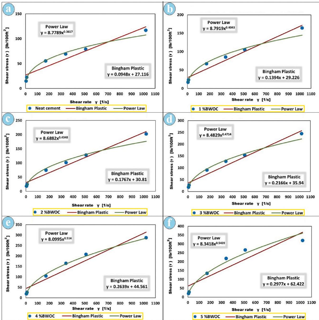
Fig. 8. Shear stress vs. shear rate for the cement samples containing (a) 0 %BWOC of APCP, (b) 1 %BWOC of APCP, (c) 2 %BWOC of APCP, (d) 3 %BWOC of APCP, (e) 4 %BWOC of APCP, and (f) 5 %BWOC of APCP.
