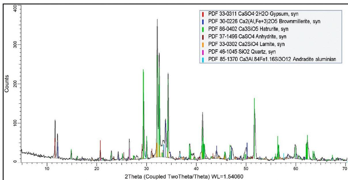
Fig. 5. XRD analysis results for the neat Class G cement.
