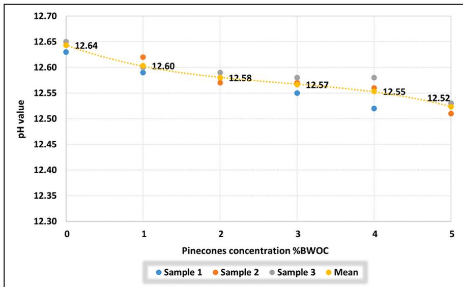
Fig. 15. pH values of the cement samples at different concentrations of APCP.
