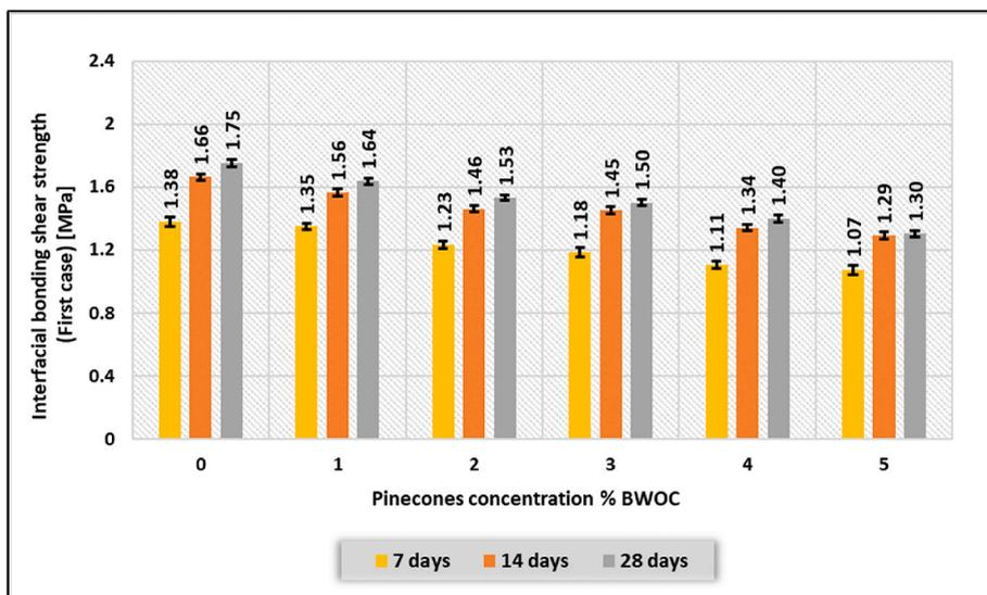
Fig. 19. Interfacial bonding shear strength of the cement samples at different concentrations of ACP for first case.
