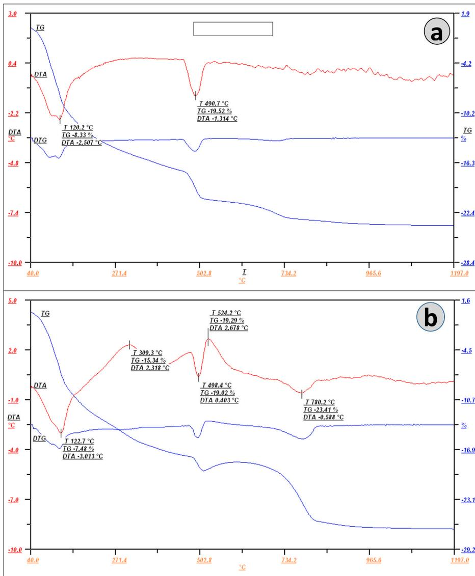
Fig. 22. TG/DTA curves of (a) neat cement and (b) cement containing 5 %BWOC of APCP.
