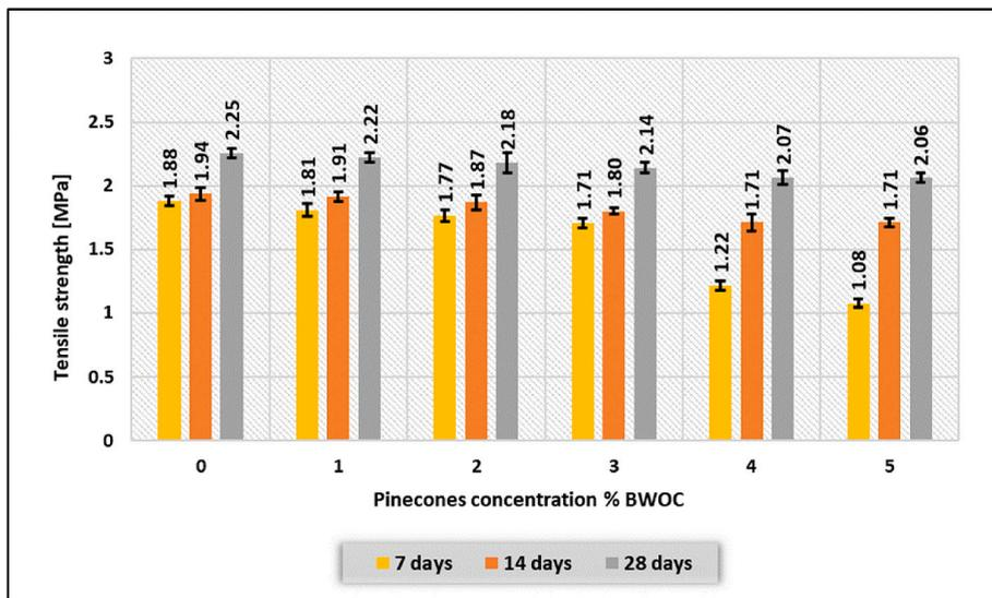
Fig. 17. Tensile strength (TS) of the cement samples at different concentrations of APCP.
