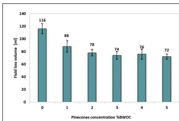
Fig. 10. API fluid loss volume of the cement slurry at different concentrations of APCP.
