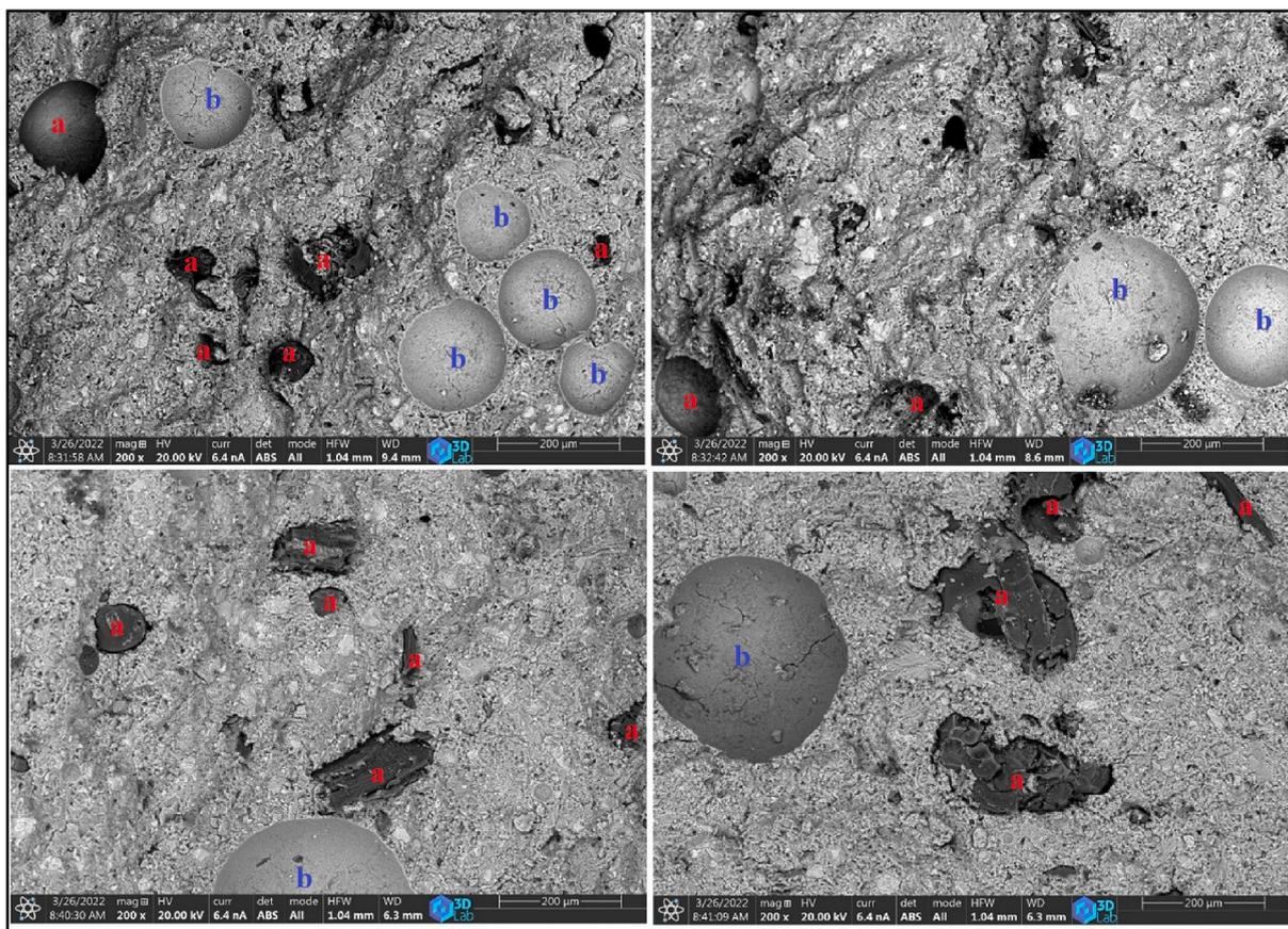
Fig. 23. SEM images of the broken face of the solid cement sample shown (a) APCP particles, and (b) pores.
