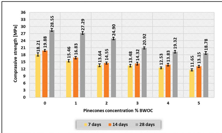
Fig. 16. Unconfined compressive strength (UCS) of the cement samples at different concentrations findings for compressive strength, of APCP.
