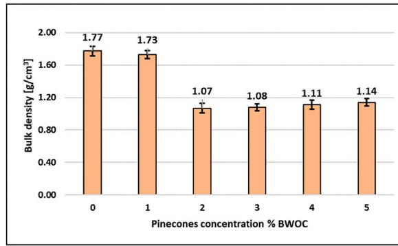
Fig. 14. Bulk density results with the addition of increasing concentrations of APCP.
