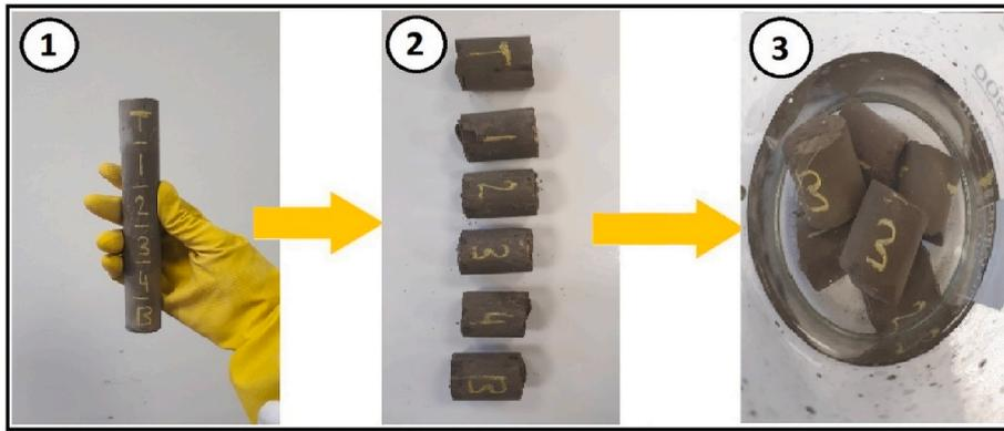
**Fig. 6.** Sedimentation test (1) the cement sample before cutting (2) the segments of the cement sample after cutting (3) segments immersed in a water bath.
