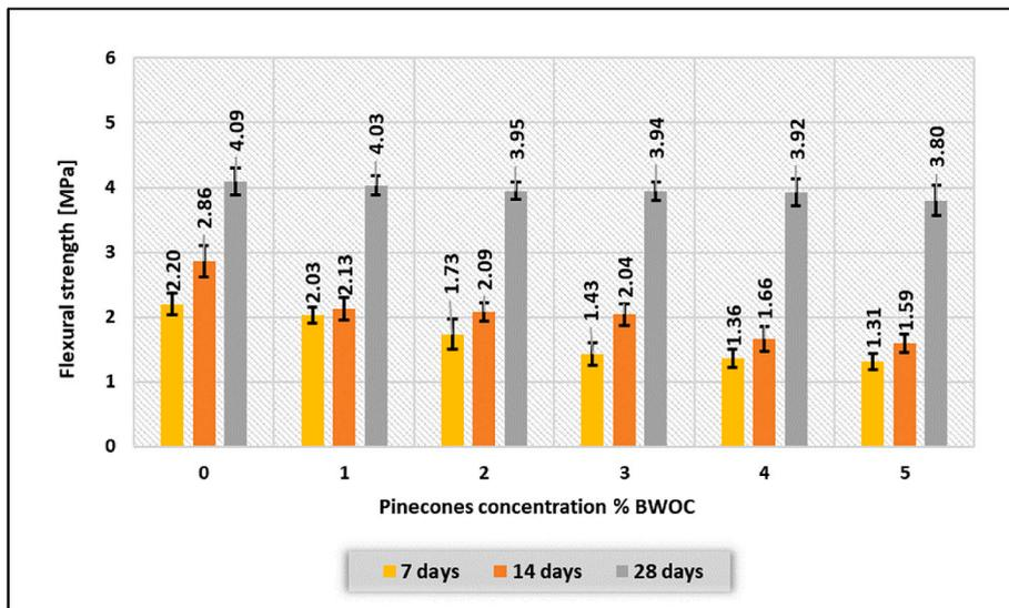
Fig. 18. Flexural strength of the cement samples at different concentrations of ACP.
