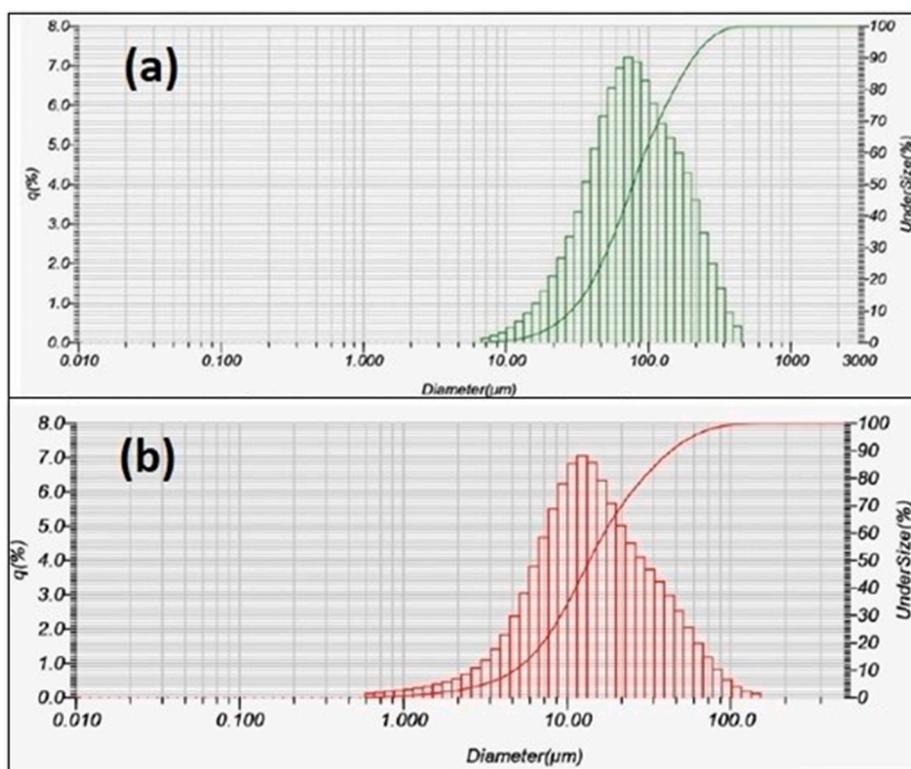
Fig. 2. The particle size distribution of (a) the APCP and (b) the neat cement powder.
