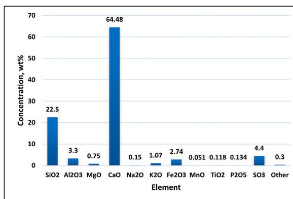
Fig. 4. Elemental composition of class G well cement by using XRF analysis.
