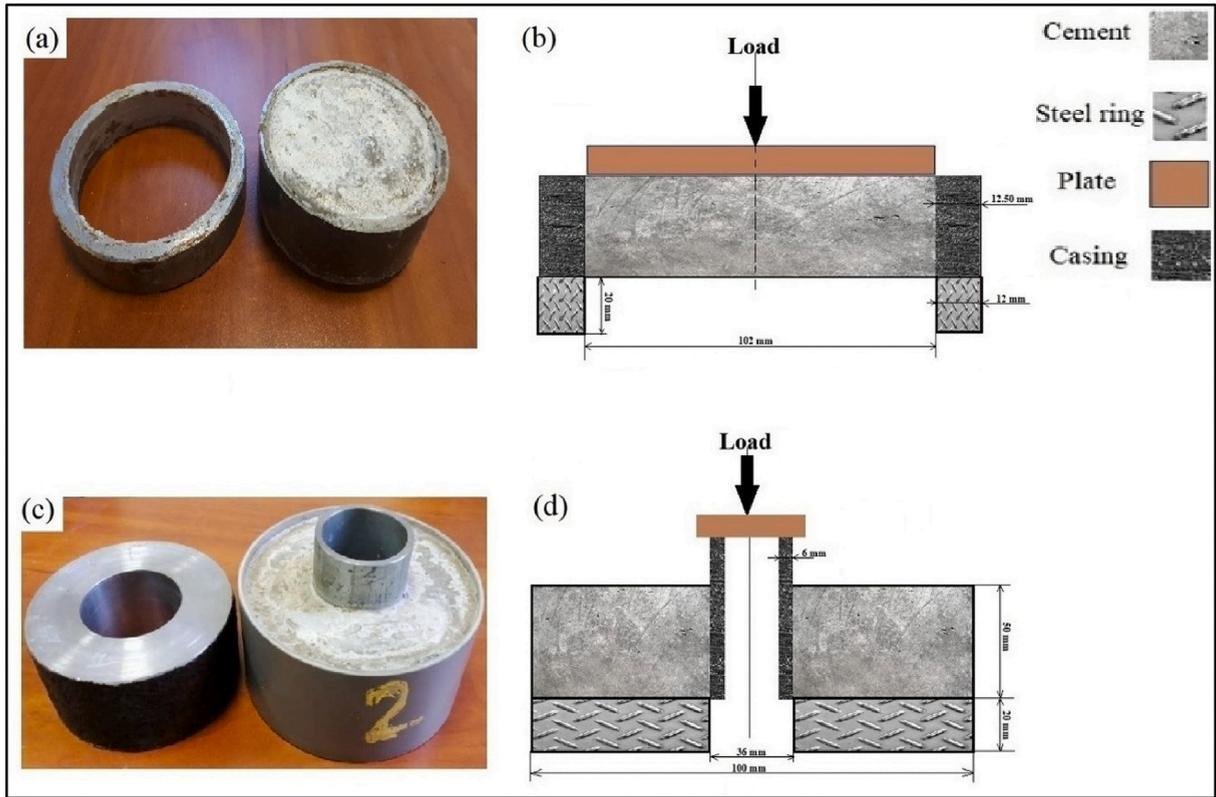
Fig. 7. Interfacial bonding shear strength in two cases: the first case (a, b) and second case (c, d).
