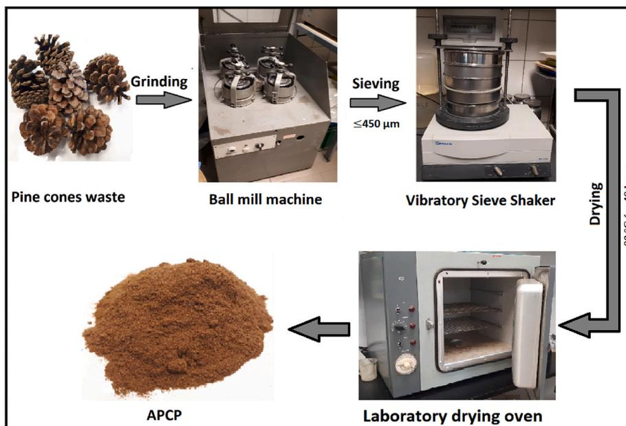
Fig. 1. Manufacturing process to produce ACP.
