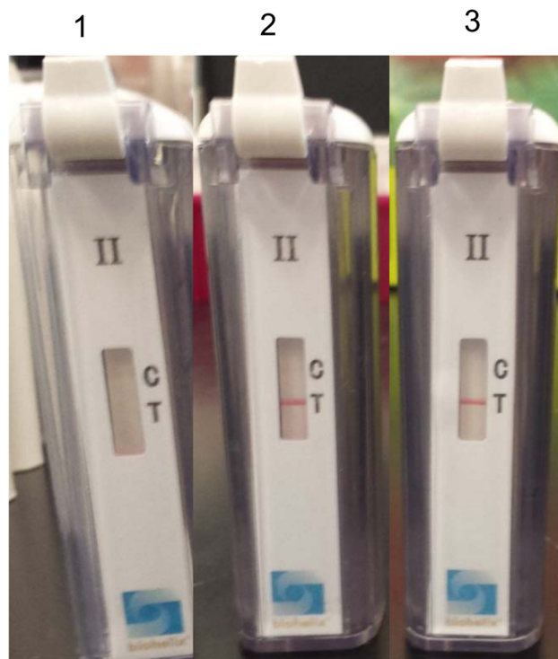
Fig 6. Evaluation of RPA-nfo assay using XCP cassette. The RPA-nfo assay for both 17 kDa gene of R. typhi and 47 kDa gene of O. tsutsugamushi was performed as described in Materials and Methods. Upon completion of the assay, the reaction tube was transferred to the cassette and the cassette was closed. The appearance of a red line along the T mark indicated the positive detection of FAM labeled probe. Cassette 1 reaction mixture contained no DNA template and complete primer sets for 47 kDa gene and 17 kDa gene with FAM labeled probes. Cassette 2 was the same as cassette 1 with the addition of 350 copies of O. tsutsugamushi DNA. Cassette 3 was the same as cassette 1 with the addition of 350 copies of R. typhi DNA. *Note: As mentioned previously, no C line was expected because there are no DIG-labeled primers in the RPA reactions, as these cassettes were initially designed for the LAMP assay.
