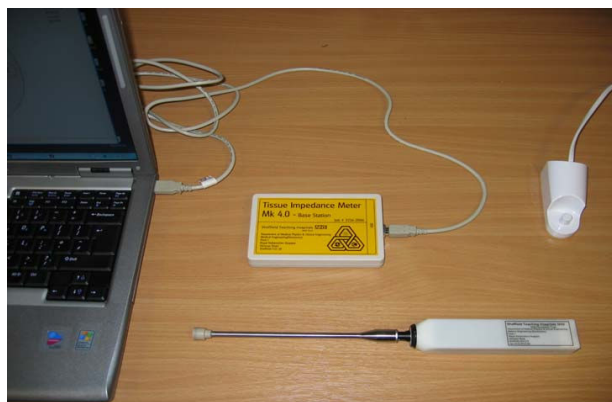
Figure 2 Setup of Sheffield Mark IV Impedance Measurement system.
