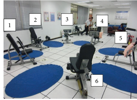
FIGURE 1: The resistance training facilities: [1] chest press/row, [2] hip abduction/adduction, [3] shoulder press/lateral pull-down, [4] leg press/curl, upright row/press, [5] biceps curl/triceps extension, and [6] leg extension/curl, side bend machines.
