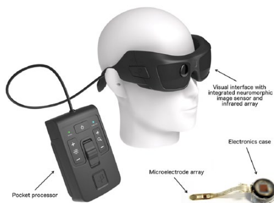
Figure 2. The Intelligent Retinal Implant System (IRIS) II. Source: Adapted from Pixium Vision S.A., Paris, France.
