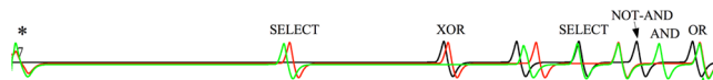
Figure 7. Spikes recorded at the electrode E_7 . The moment of initial stimulation is shown by ‘*’. Black lines show the potential when the network was stimulated by input pair (01), red by (10) and green by (11).
