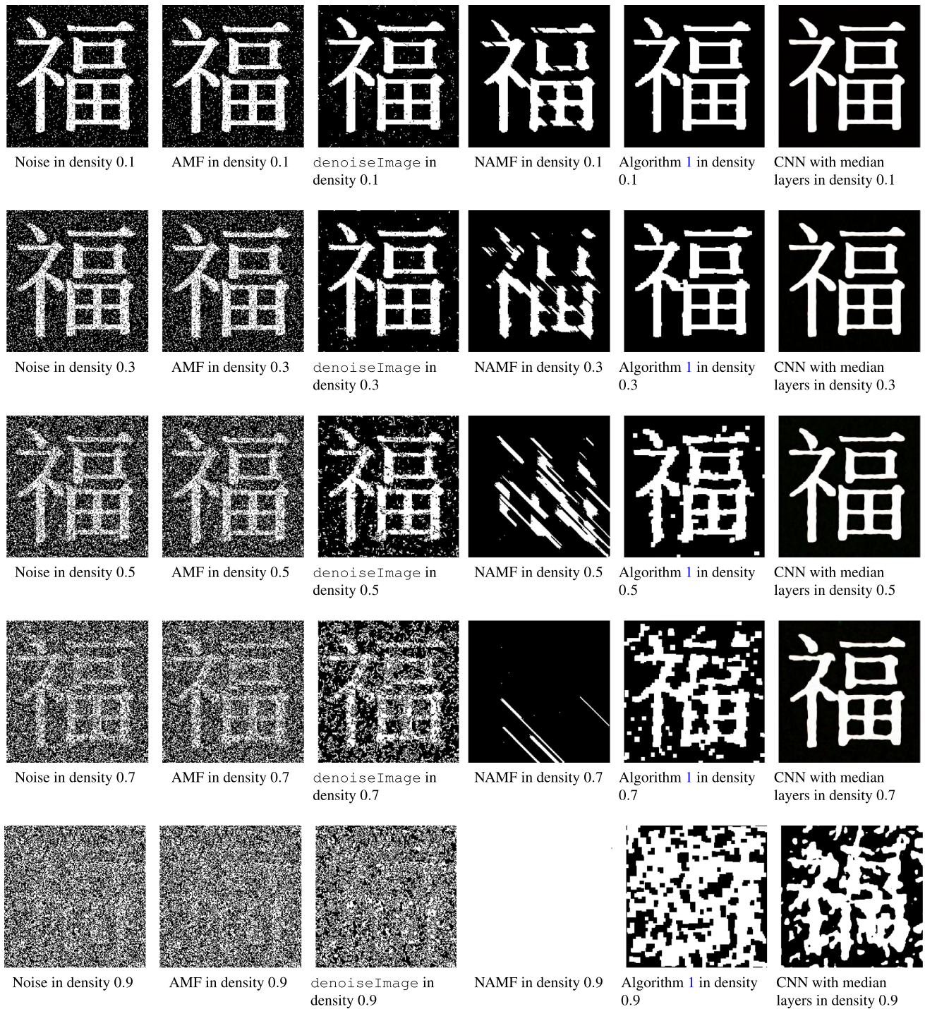
Figure 6. Conceptual images with salt and pepper noise and the results of different denoised algorithms: AMF 29 , denoiseImage, NAMF 31 , Algorithm 1, and CNN with median layers 30 . The parameters for Algorithm 1 are MaxIter=10 and Sisetol=5. Figure 5a is the ground truth image of the experiment.
