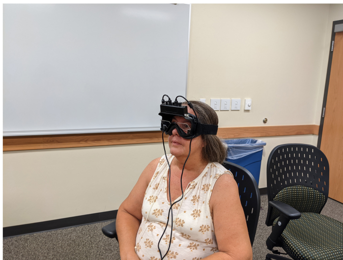
Figure 2 Subjects with goggles. Subject seated in front of TV screen with goggles placed so pupils are captured by the infra red cameras in the goggles.
