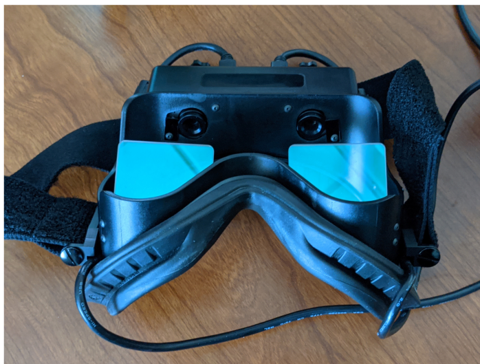
Figure 1 Goggles with infra red camera. The goggles include an infrared camera for each eyes so the pupil diameter of each each is measured.
