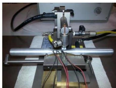
Figure 3. Example specimen during welding of the thermocouple with a lateral surface.
