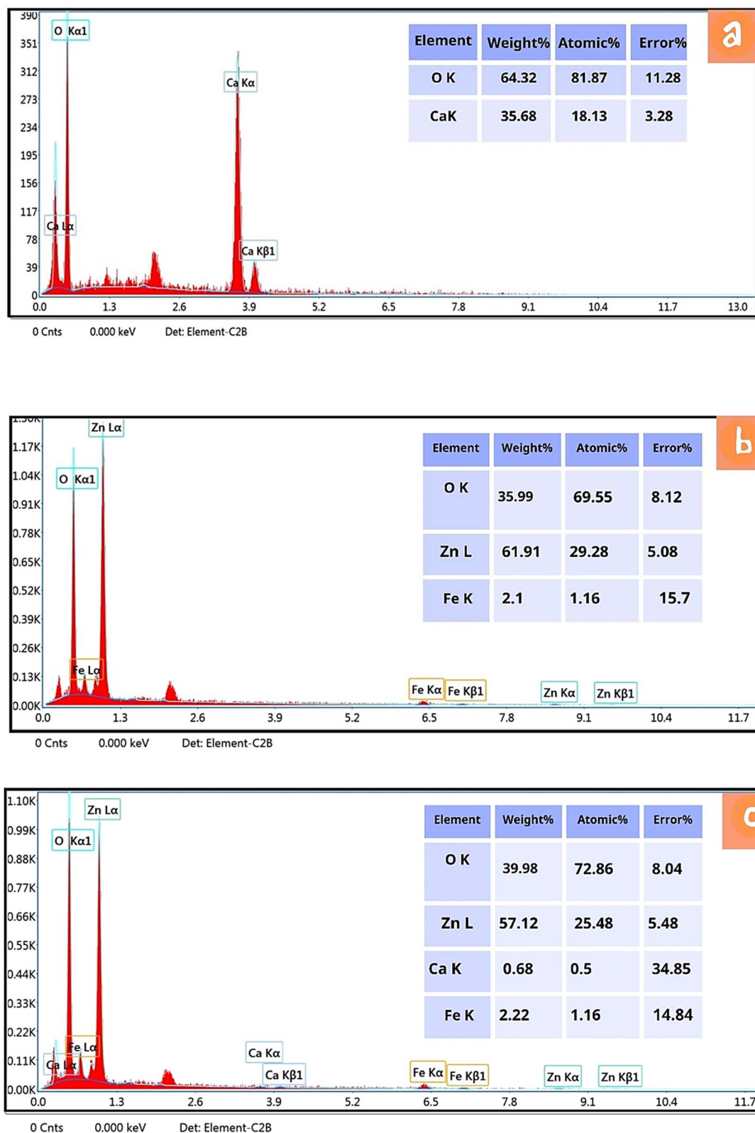
Fig. 1 EDX of (a) CaO, (b) ZnFe-LDH, (c) CaO/ZnF-LDH.
