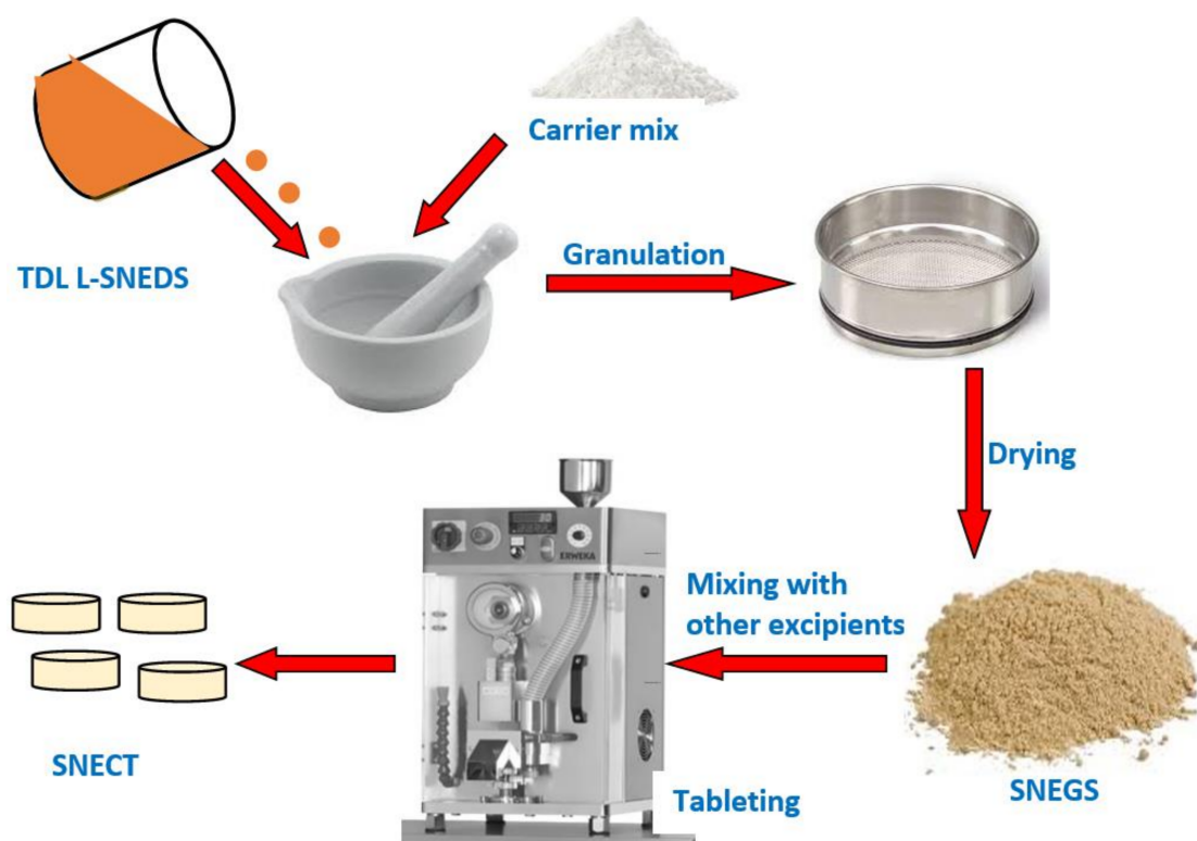
Figure 1. Preparation steps of tadalafil-loaded self-nanoemulsifying chewable tablets (SNECT).
