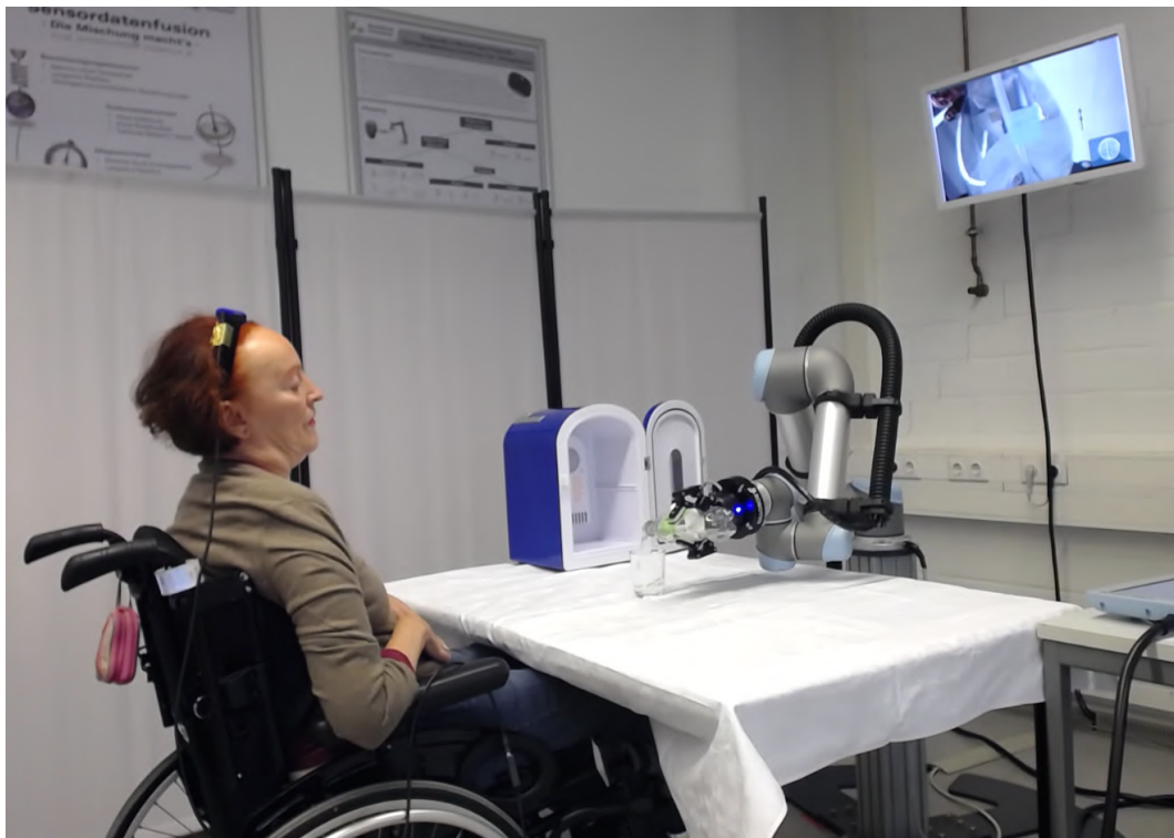
Figure 7. The test subject uses AMiCUS 2.0 to pour water from a bottle into a glass.
