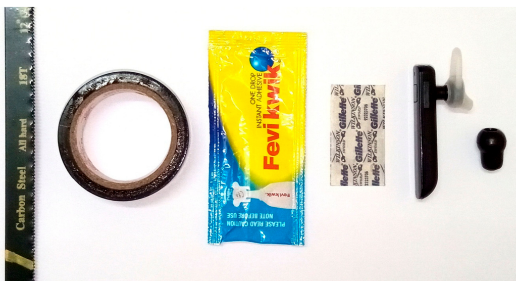
Figure 2. Materials used to transform a Bluetooth headset to a wireless phonocardiograph (From left to right: Hacksaw blade, poly vinyl carbonate (PVC) tape, instant adhesive, blade, Bluetooth headset, stethoscope ear knob).
