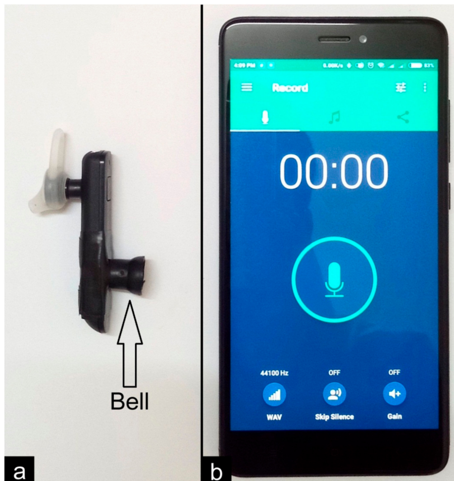
Figure 4. Developed wireless phonocardiograph (WiPCGh). (a) Modified Bluetooth headset; (b) mobile phone with audio recording software (Parrot user interface).
