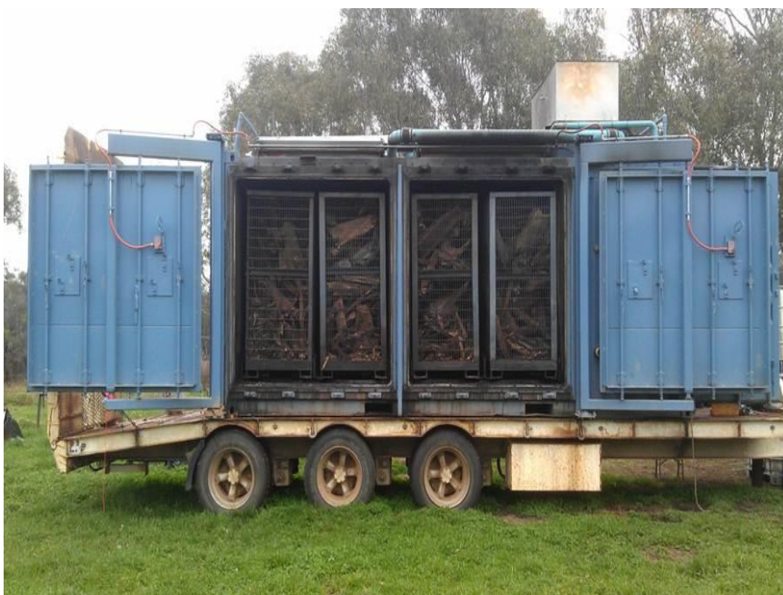
Figure 2. CharMaker commercial facility used for pyrolysing biosolids in this study.
