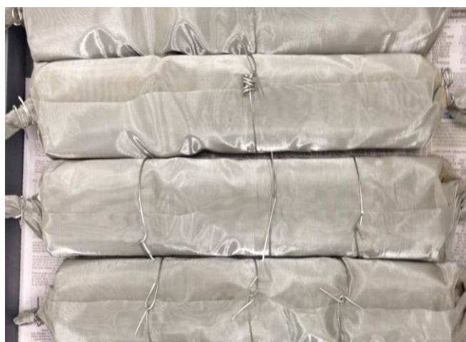
Figure 1. Stainless-steel mesh rolls with biosolids inside.
