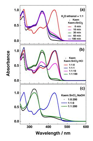
**Figure 4.** Effects of addition of water, acid, and base on the stability of the  $[Sn(II)(Kaem)_2]$  complex. Absorption spectra of solution of 50 µM HKaem and 50 µM SnCl<sub>2</sub> measured (**a**) in water:ethanol = 1:1, v/v, and in ethanol by addition of (**b**) 50, 500, and 5000 µM hydrochloric acid and (**c**) 1 mM sodium hydroxide. Absorption spectra of 50 µM HKaem alone under the same conditions is indicated by a dashed line for comparison.
