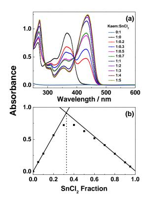
**Figure 2.** Determination of the Sn:Kaem ratio. (**a**) Absorption spectra of 50  $\mu$ M HKaem, 50  $\mu$ M SnCl<sub>2</sub>, and solutions of 50  $\mu$ M HKaem addition of SnCl<sub>2</sub> in varying ratio (1:0.2–1:5) in ethanol. (**b**) Job's plots of absorbance at 430 nm obtained by mixing solutions of HKaem and SnCl<sub>2</sub> with total concentration of 50  $\mu$ M in HKaem:Sn(II) molar ratios varying from 9:1 to 1:9.
