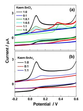
**Figure 9.** Cyclic voltammograms of 100  $\mu$ M HKaem alone and (**a**) 100  $\mu$ M SnCl<sub>2</sub> and solutions of 100  $\mu$ M HKaem with 10, 50, 100, and 200  $\mu$ M SnCl<sub>2</sub>, and (**b**) 100  $\mu$ M Sn(OAc)<sub>2</sub> and solutions of 100  $\mu$ M HKaem plus 100  $\mu$ M Sn(OAc)<sub>2</sub>. All samples were in ethanol relative to 50  $\mu$ M ferrocene with 0.1 M sodium perchlorate, NaClO<sub>4</sub>.
