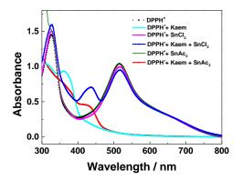
**Figure 7.** Absorption spectra of 100 μM DPPH<sup>•</sup>, 100 μM DPPH<sup>•</sup> plus 100 μM HKaem, 100 μM DPPH<sup>•</sup> plus 100 μM SnCl<sub>2</sub>/Sn(OAc)<sub>2</sub>, and 100 μM DPPH<sup>•</sup> plus 100 μM HKaem + 100 μM SnCl<sub>2</sub>/Sn(OAc)<sub>2</sub>. Ethanol was used as the solvent.
