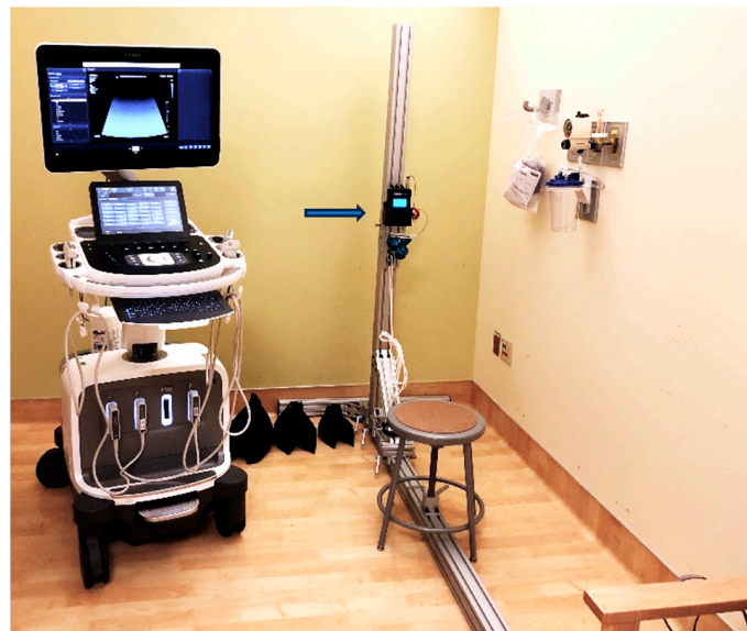
Figure 2. Custom-designed apparatus for applying loads at different upper extremity positions. The aluminum vertical post allows the height of the pulley to be adjusted to ensure the force vector is in line with the lower arm, and a load cell with a digital display (arrow) was used to measure the applied forces.
