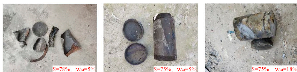
Figure 15. The effect of solid content and Al on response to slow roasting composition changes on the response of slow cook-off [63].
