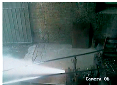
Figure 11. Standard engine test diagram for 5% Al and 73% AP [47].
