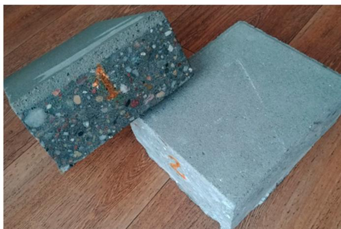
**Figure 1.** Photocatalytic concrete paving block studied in the research with a novel test method.
