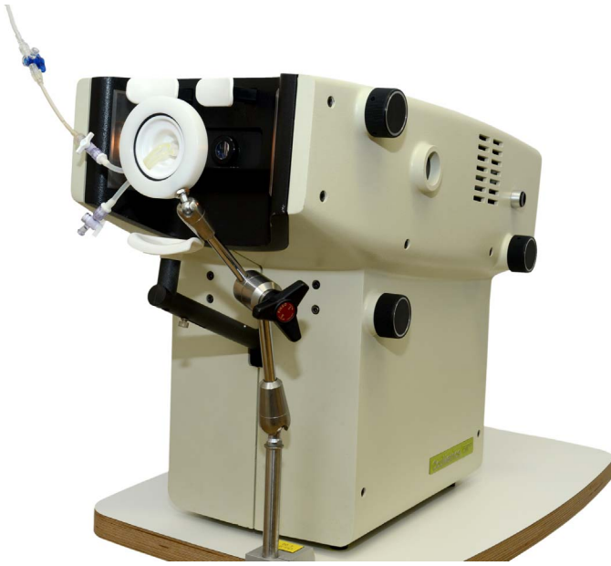
Figure 2. Optical head of the Fluorotron Master FM-2 fluorophotometer fitted with multijoint adapter accommodating an artificial anterior chamber with two irrigation ports attached to the base. The cornea (mounted on the artificial anterior chamber's tissue pedestal and therefore not visible from this perspective) is aligned with the lens and the centering is checked via the alignment window in the side housing.
