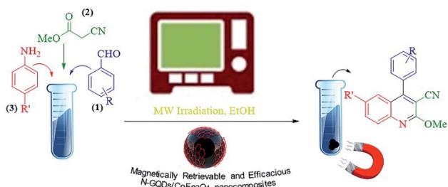
Scheme 1 MW-assisted synthesis of quinoline-3-carbonitrile frameworks.
