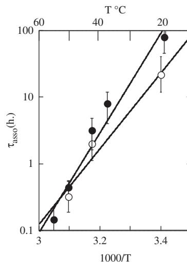
**Figure 4.** Sms half formation times vs. temperature of  $C_7GC_4$  (black circles) and  $C_4GC_7$  (open circles) 0.3 mM solutions in the NAP buffer at pH 4.6. The activation energies related to sms formation,  $143 \pm 40$  and  $110 \pm 25$  kJ/M are comparable.
