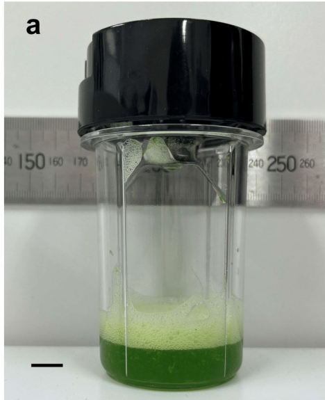
Fig. S2. Plant tissue homogenized in CTAB by coffee-bean blender for 40 seconds. a. Whole view. b. Zoomed in view. The scale bar is 1 cm.
