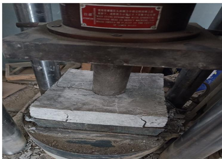
**Figure 3.** Punching strength setup.
