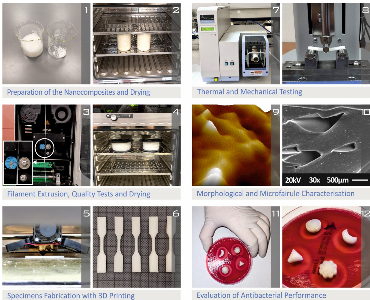
Figure 1. Presentation of the overall procedure followed for the preparation, measurement, and characterization of PA12/AgDANP nanocomposites: (1) matrix material and filler powder; (2) after the mixture of the matrix material and the nano-filler, nanopowders are dried; (3) the filament extrusion process; (4) the filament drying process; (5) specimens' 3D printing process; (6) tensile testing of specimens; (7) investigation of nanocomposites' thermal properties in the thermogravimetric analysis device; (8) flexural testing of the manufactured specimens; (9) filament surface roughness investigation in the atomic force microscopy device; (10) investigation of specimens' surface morphology in scanning electron microscopy device; (11,12) investigation of the antibacterial performance of the nanocomposites for E. coli bacterium with the agar well diffusion screening process.
