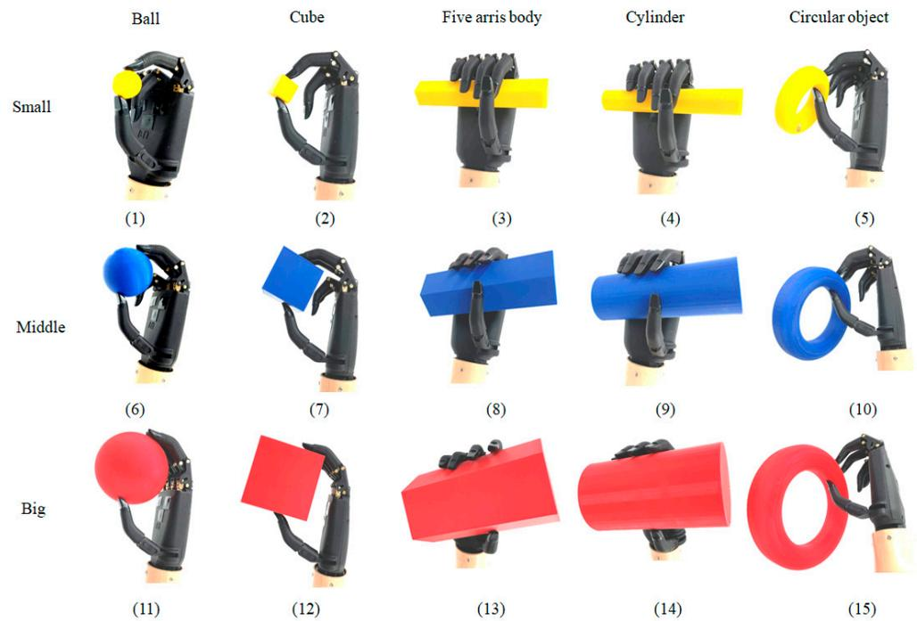
**Figure 15.** Grasp test of different objects of BIT hand C.
