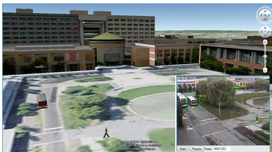
Figure 14 3D Town outdoor moving object tracking and recognition: video from surveillance camera (bottom-right inset).
