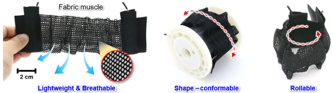
Figure 1. Breathable, light, soft, and flexible fabric muscle.
