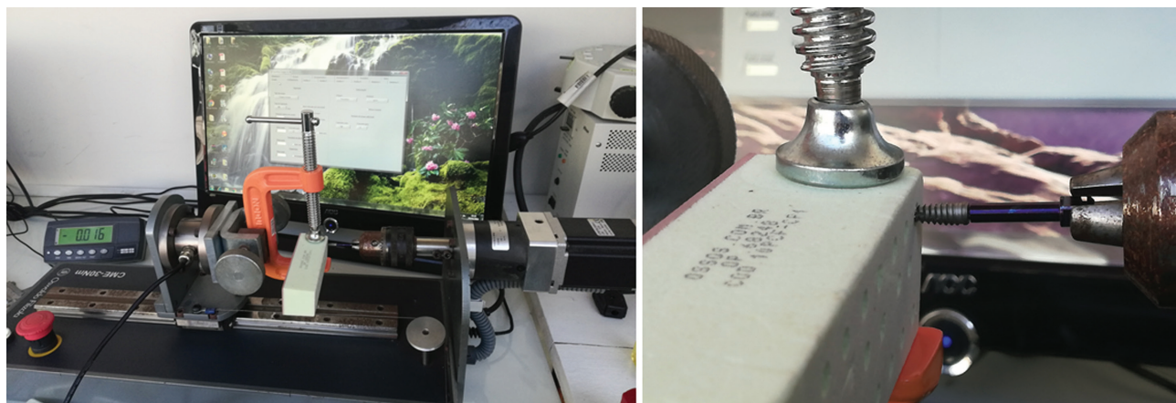
Figure 5: Image of the machine used for implant insertion and torque measurement
