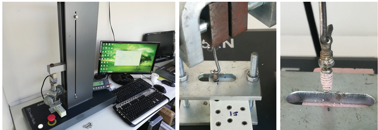
Figure 6: Image of the machine and dispositive used for the pullout test
