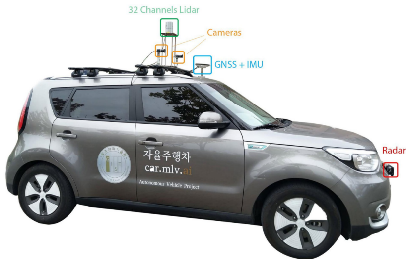
Figure 1. Our KIA-Soul EV is equipped with two FLIR cameras, a 3D 32-laser scanner and a GPS/IMU inertial navigation system [24] (Best viewed in color).
