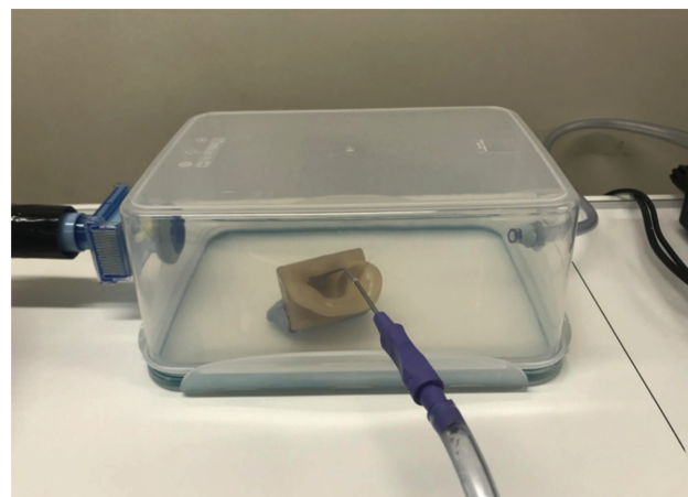
Figure 2. Suction performed through a port in the chamber.
