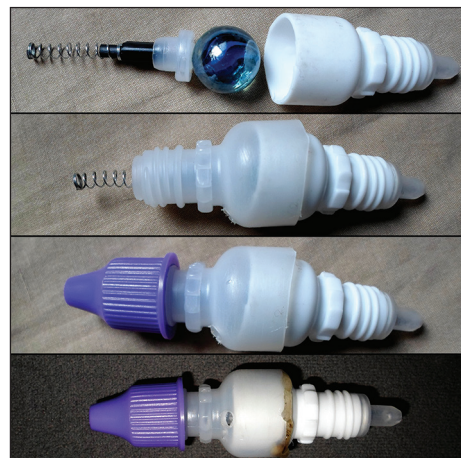
Figure 3: Assembly of the pressure release valve
