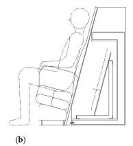
**Figure 1.** (a) Chair-type whole body counter at Fukui Prefectural Hospital. (b) Schematic drawings of the two NaI(Tl) detectors aligned alongside and horizontally in the chair.
