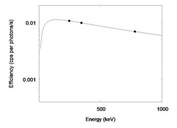
**Figure 6.** Efficiency curve derived from the  $^{152}$ Eu point source measurement. Rigid circles indicate calculated values from measurement. The solid line shows the weighted least-squares fitting result.
