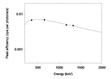
**Figure 5.** Efficiency curve derived from the NIRS BOMAB phantoms. Rigid circles indicate the measurement results. The solid line shows the least-squares fitting result.
