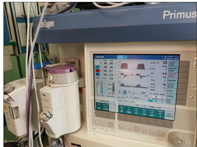
Figure 1: Dräger Primus Anaesthesia workstation showing the halothane red rectangle after asthalin puffs given via the endotracheal tube
