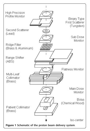
SOBP was 6 cm in length. A total of 107 Gy was delivered in 10 sessions of irradiation at the SOBP center, and ranged from 2 to 20 Gy in one session. The ICDs were monitored during proton beam irradiation in order to detect the alarm sound that is produced by the device to notify the occurrence of serious soft errors.
