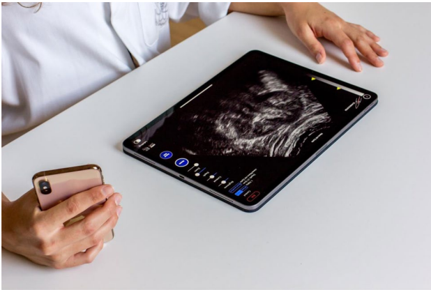
Fig. 2 The setup of the simulation. The ultrasound simulation was displayed on a tablet (serving as a display), the control was implemented by a smartphone (serving as a virtual probe) with the Scanbooster Control app installed on it. The two devices were subsequently connected via Bluetooth. By moving the smartphone in space, the corresponding ultrasound image was realistically calculated by the app and displayed on the tablet in real-time
