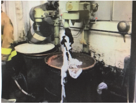
FIGURE 1: The scene of the accident. The patient's clothing was entrapped and wound around the mixing rotator.
