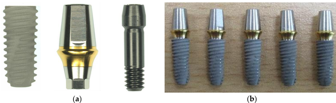
Figure 1. Component of implant systems for static and dynamic experiments. (a) Fixture (GSTA5620) with 10 mm of length and 4.5 mm of diameter, the abutment (TS3S5011S) and abutment screw (GSABSS) and (b) assembled implant specimens.
