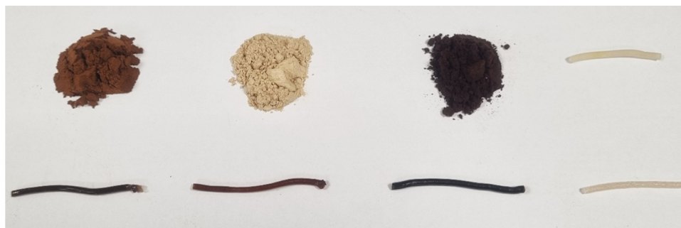
Figure 2. (Top row, left to right) SC, BSG, SCG powder after sieving and TPS filament (second row, left to right) PLA-SC (15%), PLA-BSG (15%), PLA-SCG (15%), and PLA-TPS (15%).
