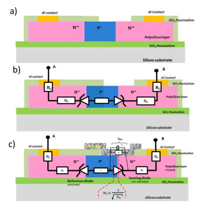
**Figure 3.** Basic cross section of Zener diode-based platform: (a) the overall structure of a single element; (b) the electrical equivalent circuit; (c) the electrical equivalent circuit after the sensitive MOX layer.
