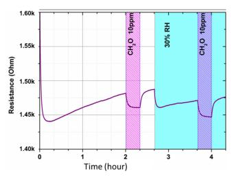
**Figure 12.** Static test: resistance measurement versus time under various atmospheres. Injection of 10 ppm of formaldehyde under dry air and then under humid air (30%RH).
