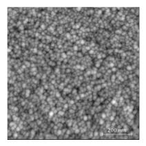
**Figure 5.** AFM image of a 25 nm thick ZnO:Ga.
