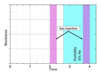
Figure 11. Static test protocol: equivalent resistance measurement versus time under various atmospheres.
