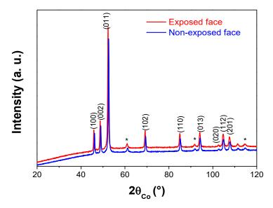
**Figure 2.** Experimental XRD patterns recorded on the directly exposed (red line) and non-exposed (blue line) to plasma implantation Ni pellet, within grazing conditions. Both were successfully indexed within the hexagonal Ni<sub>2</sub>H structure (ICDD n° 98-020-1088). The small peaks marked by an asterisk correspond to the diffraction planes of the cubic Ni structure (ICDD n° 98-004-3397).
