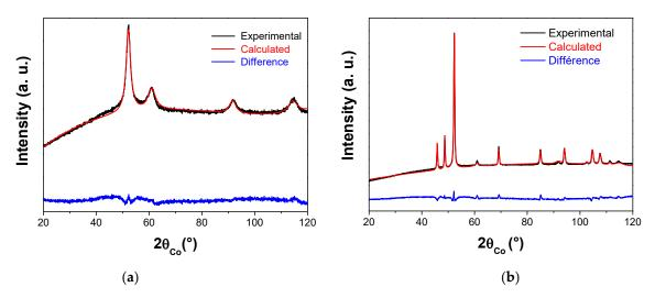
**Figure 1.** Experimental (black scatter) and calculated (red line) X-ray diffraction (XRD) patterns of polyol-made (**a**) and plasma treated (**b**) Ni powders. The residue, defined as the difference between the experimental and calculated diffractograms, is given (blue line) to illustrate the fit quality, with a Bragg reliability factor *R*<sub>B</sub> ranging between 1.5 and 2.0.
