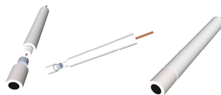
Scheme 1 Architectural illustration of the working electrode, showing a disk-shaped miniature neodymium magnet behind the glassy carbon.
