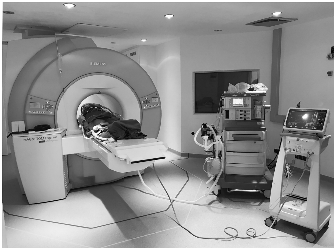
Fig 2. Setup of anesthesia equipment in the iMRI scanner. The MR-capable ventilator (Dräger Fabius MRI, Drägerwerke, Lübeck, Germany) is positioned outside the 30 mT area (dark line) while the monitoring hardware has to be kept outside the 20 mT area (light yellow line).
