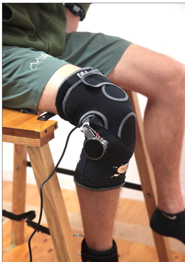
Figure 3. Subject sitting on the platform and connected to the linear actuator. The electro goniometer is shown on the knee.
