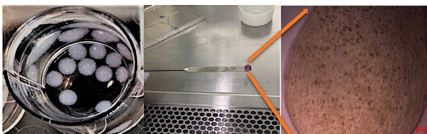
Figure 1. Alginates beads crosslinked with CaCl 2
