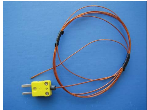
Figure 2: Type K flexible thermosensor
