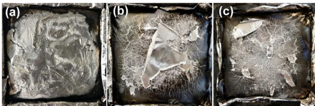
Figure 3. Digital photos of residues after cone calorimeter tests for PLA (a), PLA3 (b), and PLA4 (c).
